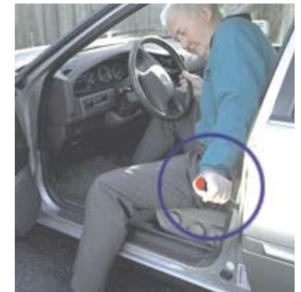
Insert the Handybar® into the U-shaped striker plate located on the driver and passenger-side door frames of the vehicle.
