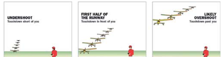
FIGURE 8 Reducing power and altitude prior to the final turn sets up a lower approach, which makes judging when to idle the engine a lot easier.
